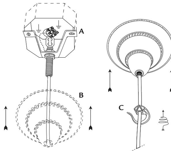
5. Screw the hook **C** onto the nipple and tighten securely.
